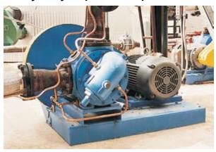
For emulsions, filled asphalts, high pressure and refinery applications, Viking® Heavy Duty jacketed pumps feature a thrust bearing that fixes the rotor position in the head, so users can set precise clearances and compensate for wear over time. Options for these durable pumps include:
